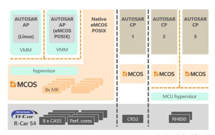
MK: microkernel of multikernel VMM: virtual machine monitor Perf. cores: performance cores CR/RH850: safety cores
